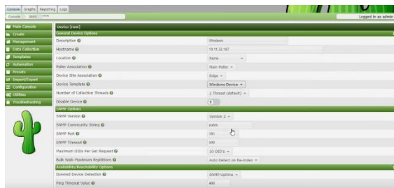
Gambar 4.5 Seting Monitoring SNMP
