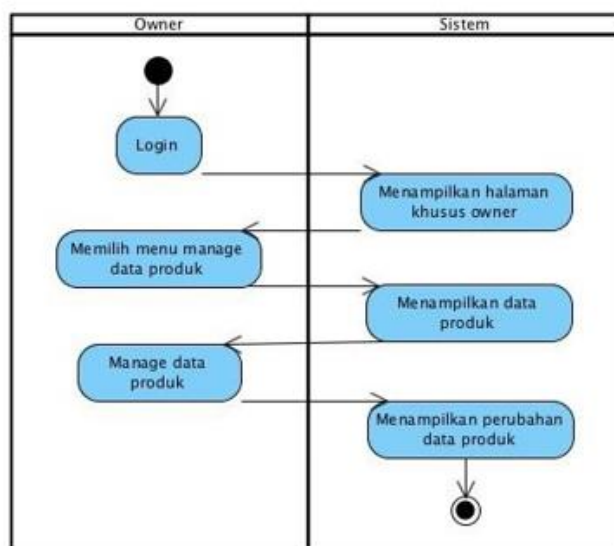
Gambar 10. Activity Diagram Use Case Manage Data Produk
